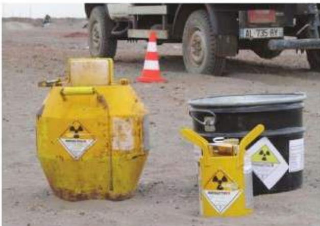
Figure 21: Neutron and Density sources contained in shields
